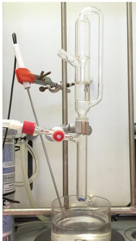
**Figure 1.** A typical reaction setup for olefin metathesis using XiMoPac catalyst system
